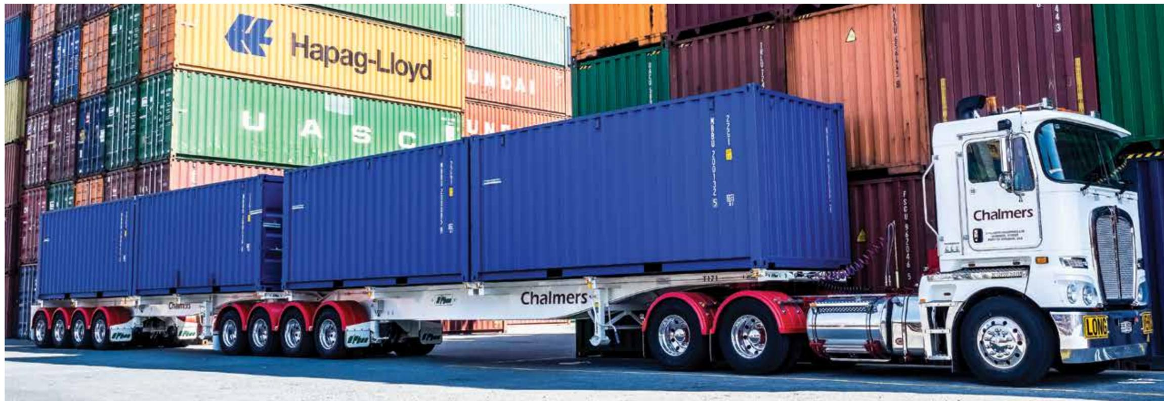
TO INCREASE THE EFFICIENCY OF ITS CONTAINER MOVEMENTS AT THE PORT OF BRISBANE, TRANSPORT COMPANY **CHALMERS INDUSTRIES** HAS WORKED WITH **O'PHEE TRAILERS** TO DEVELOP AN APPROVED QUAD-QUAD SUPER B-DOUBLE.
