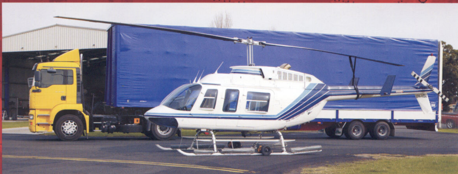
The 14.6 metre long and 4.6 metre high O'Phee trailer is specced with a BPW tandem axle air suspension system, chosen for its smooth ride characteristics and Netcap Load Protection System.
